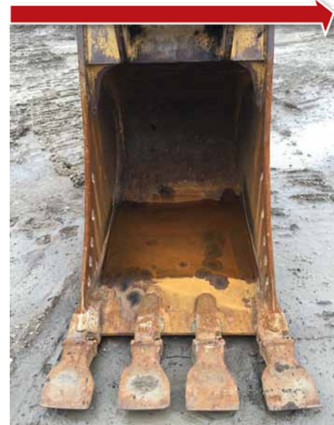
Without a straight bar attachment, the paddle teeth on this bucket can easily rupture or puncture a utility line.
